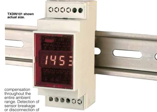
input leads, forces the output to a pre-defined up/down scale value. The unit continuously monitors the sensor and automatically returns to normal operation mode when the sensor is recovered. The TXDIN101 is housed in a plastic enclosure mounted on a standard DIN rail. Special red filter is provided for optimal view.
