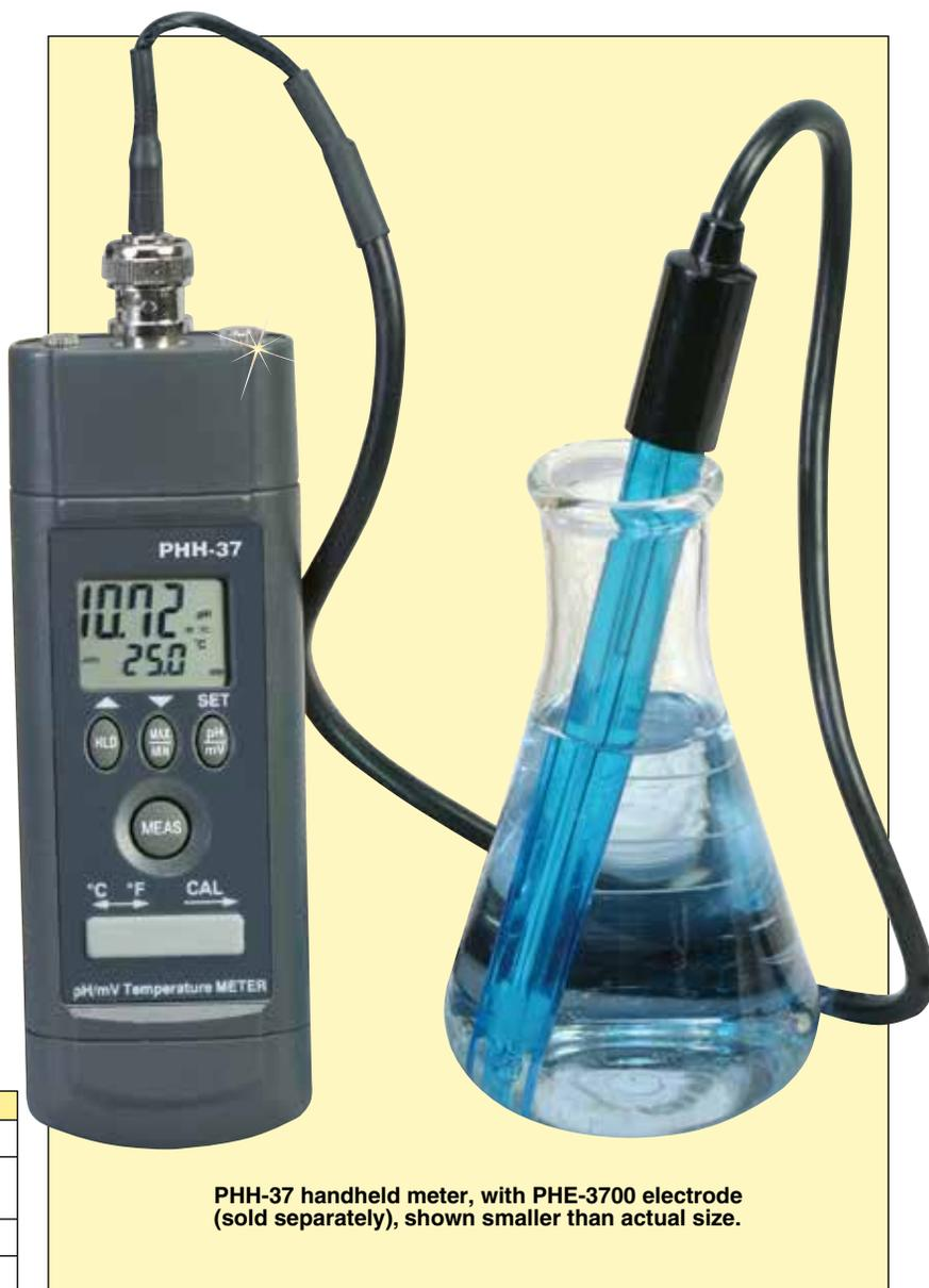
PHH-37 handheld meter, with PHE-3700 electrode (sold separately), shown smaller than actual size.
