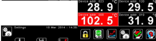
Display and configure all 6 channels individually or simultaneously. Displays channels in red in alarm condition.
