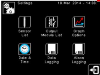
Configure options for each sensor and the TSD600 itself via the touch screen interface.
