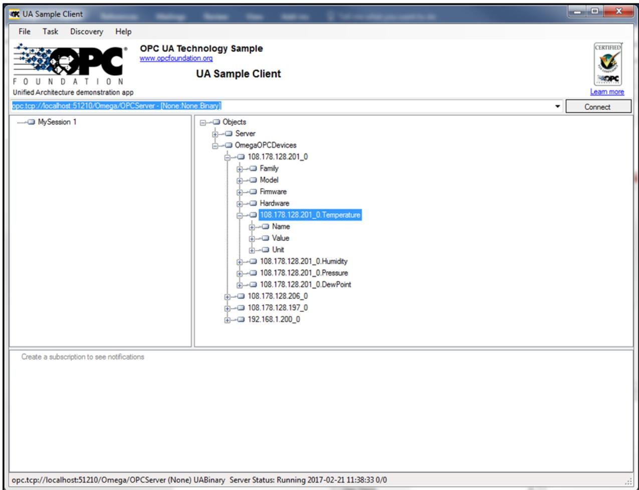
Figure 48: OPC UA Sample Client tree structure
