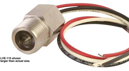
switches utilize a strong, glass prism fused to a carbon steel or housing to easily monitor vessels pressurized up to 2500 psi. Their compact package size makes them the ideal candidate for monitoring the small, pressurized vessels found in HVAC, refrigeration and hydraulic applications. They are most commonly used for low, high and intermediate level detection.
