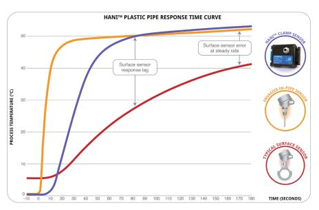
1. t63 is the time constant or response time required to reach 63.2 % of the final value after an instantaneous temperature change. t90 is the response time required to reach 90 % of the final value after an instantaneous temperature change.
