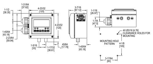
The Series DHII Digihelic® II Differential Pressure Controller takes all the features of the standard Digihelic® pressure controller and packages them in a robust NEMA
