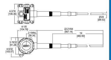
Service: Liquids, powder, and bulk materials compatible with wetted materials. Wetted Materials: 316 SS and polyvinylidene fluoride (PVDF). Temperature Limits: Ambient: -40 to 185°F (-40 to 85°C), -4 to 185°F (-20 to 85°C) with under 24 VAC/DC power supply; Process: -40 to 250°F (-40 to 121°C).
