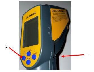
Press the "°C/F" button to toggle to °C (arrow #2)
