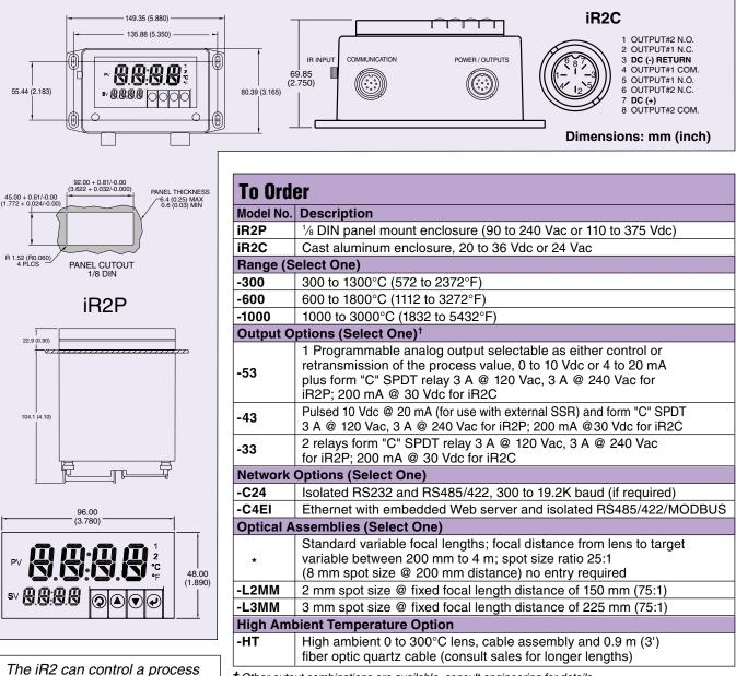
*†* Other output combinations are available, consult engineering for details. **Ordering Example: iR2C-1000-53-C4EI**, 2-color infrared temperature controller in a rugged cast aluminum enclosure, with 8 mm spot size optic lens assembly, temperature range of 1000 to 3000°C (1832 to 5432°F), programmable analog output, 1 SPDT form "C" relay, Ethernet, RS485/422/ MODBUS and **iR2-06**, 1.8 m (6') fiber optic cable [substitute for standard and 1 m (3') cable].
