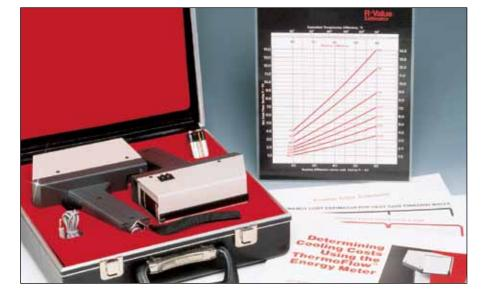
The OS-650 kit is designed to perform energy audits, insulation inspection, and general plant maintenance. The temperature meter uses a non-contact sensor to measure temperatures, while the heat flow meter is an infrared radiometer designed to detect insulation defects, estimate R-values, and measure heat loss through building walls, windows. LCD readouts show temperature and heat flow data which are readily translated into information to determine energy costs.
