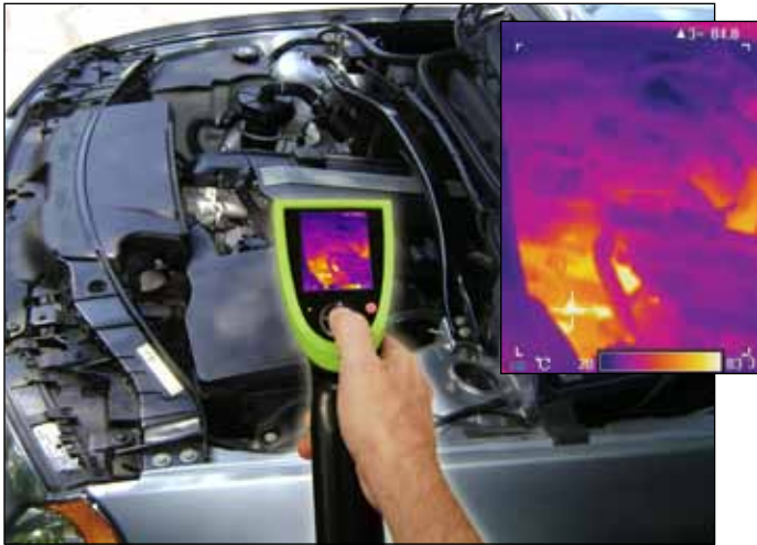
OSXL160 shown measuring an engine's surface temperature.
