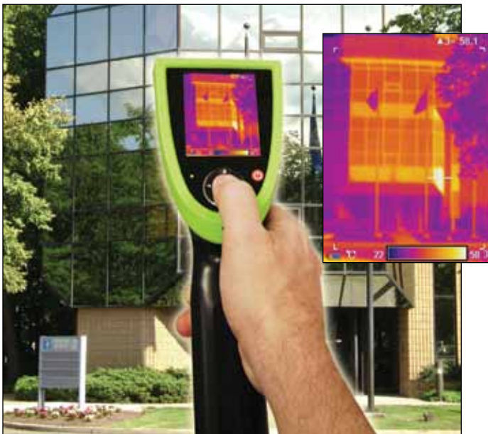
OSXL160 shown measuring temperature differences on windows and building surfaces.
