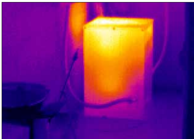
Thermal image of a power supply.
