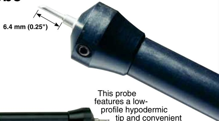
This probe features a low-profile hypodermic tip and convenient handle for short depth penetration of soft materials such as rubber. A grounded junction, 300 mm (1') of retractable cable [which stretches to 1.5 m (5)] and a subminiature male connector are standard. The handle is rated to 162°C (325°F).
