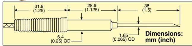
**Ordering Example:** HYP4-16-1-1/2-100-EU-48-MTP-M, RTD hypodermic probe with 1.2 m (48") leads and MPT-U male connector.
