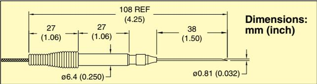
**Thermocouple Probe Model HYP2 and HYP5**
