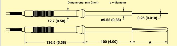
These unique leaf style surface probes are designed for instant measurement of temperature on flat surfaces.
