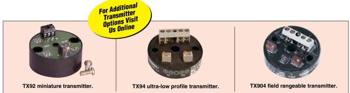
When the sensors are used in remote locations, or in environments where electro-magnetic noise is prevalent. Transmitters are a perfect choice. The transmitters shown above will convert the resistance of the RTD to a 4 to 20 mA signal (for use in PRTF-12 and -18 heads only, no transmitters available for -14 and -19 heads).
