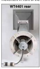
rear portion of the intake baffle has a profile design that keeps the stream uniform, while decreasing the area to a 101.6 x 101.6 mm (4 x 4") cross- section.
