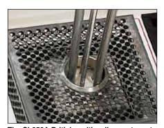
The CL950A British multi-well accepts up to 5 probes at one time and comes standard with %, %, % and two %" diameter holes. The CL950A-M metric multi-well accepts up to 5 probes at one time and comes standard with 2, 3, 4.5, and two 6 mm diameter holes.
