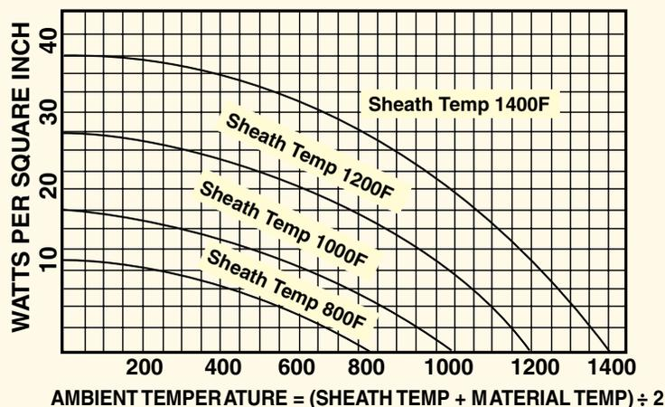
**Figure C-11- allowable watt density** of clamped-on Omegalux tubular units for various ambient temperatures and sheath temperatures.
