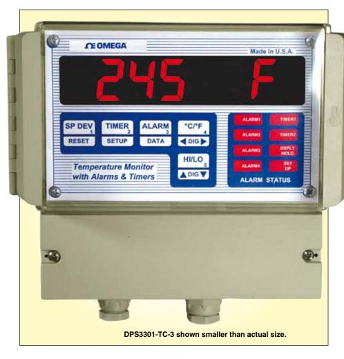
Four (optional) process alarms are available that are programmable over the entire range of selected input type. They can be configured as latching or non-latching, normally open, or normally closed. Also available are 2 optional timers that work independently or in conjunction with process limits (e.g., turning on a fan 10 minutes after limit 1 temperature is reached). The time function keeps track of process run time.
