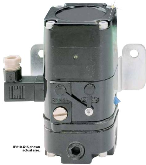
The IP210 provides a reliable, repeatable, accurate means of converting an electrical signal into pneumatic pressure. Its force balance principle is a coil suspended in a magnetic field on a flexible mount. At the lower end of the coil is a flapper valve that operates against a precision ground nozzle to create a backpressure on the servo diaphragm of a booster relay.
