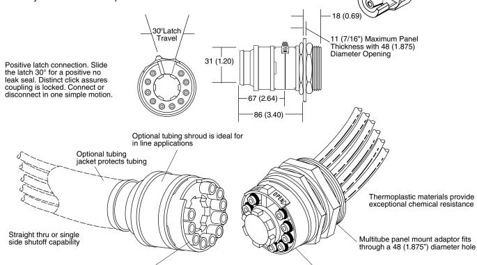
Ordering Information: Each coupling body includes ten inserts of one tube size. Purchase inserts of different sizes for replacements of original tube fittings or to mix tube sizes in the coupling. Coupling body does not include optional tubing shroud or panel mount adaptor. Specify separately depending on coupling configuration; i.e. panel mount coupling requires 1 tubing shroud, 1 panel mount adaptor. Tube-to-tube coupling assemblies require 2 tubing shrouds.
