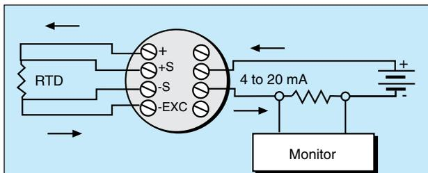
The TX1501 transmitter is designed for 3-wire RTD operation that compensates for lead resistance. The +S terminal is not connected internally. Shorting the -S and -EXC terminals provides 2-wire operation.
