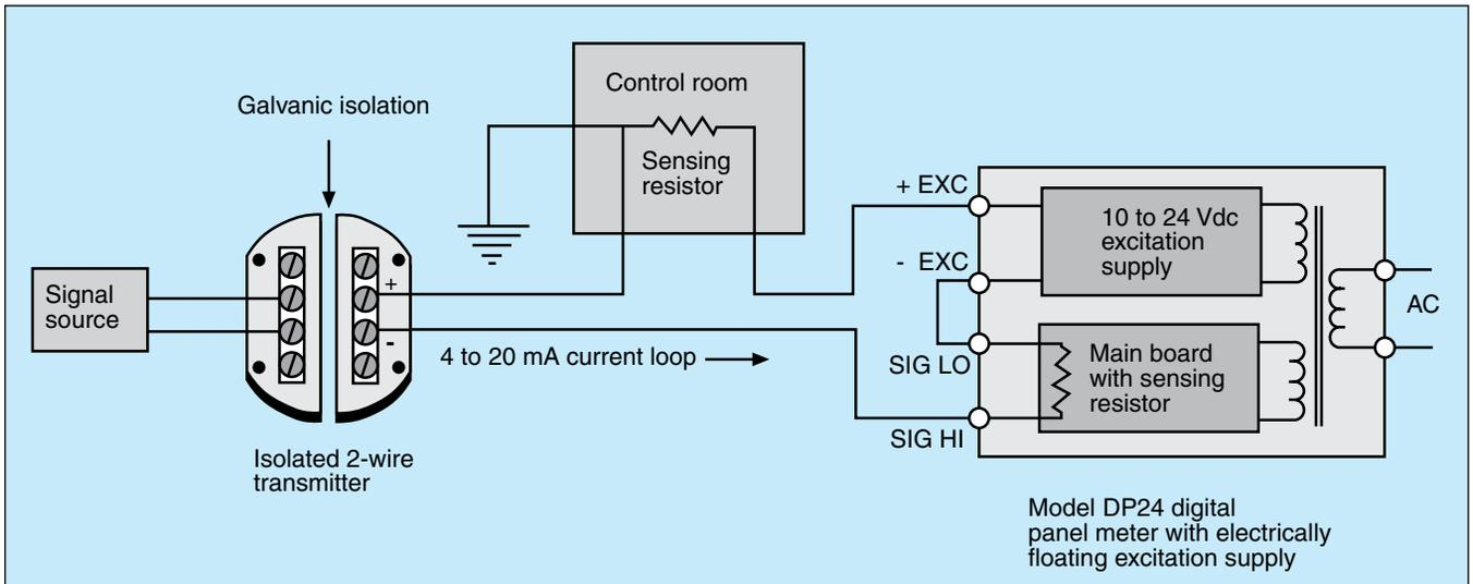
A DP24, DP25 or DP41 panel meter may be used to power the 4 to 20 mA loop, including the isolated 2-wire transmitter. One or more loads may be added to the loop, including receiving equipment in the control room. The excitation supply is electronically floating; thus, the current loop may be grounded anywhere. In addition to powering the loop, the panel meter provides a local display scaled in percent or in engineering units.
