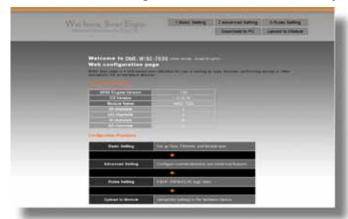
OME-WISE-7000 Series controllers are equipped with an IF-THEN-ELSE logic Rule Engine, it offers up to 36 IF-THEN-ELSE rules for users to set up the logic content. After completing rule edition and downloading rules to the OME-WISE-7000 controller, the Rule Engine will loop execute the rules in accordance with the execute order under specific conditions.
