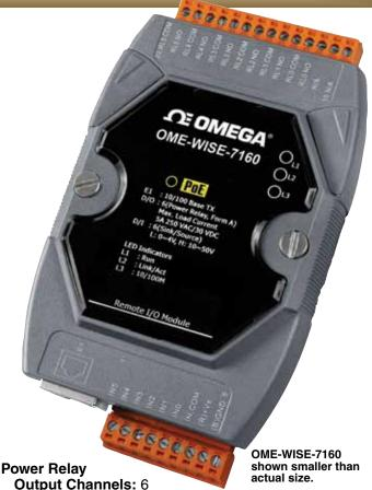
Output Type: Power relay, Form A (SPST N.O.) Operating Voltage Range: 250 Vac/30 Vdc Maximum Load Current: 5.0A/channel at 25°C
