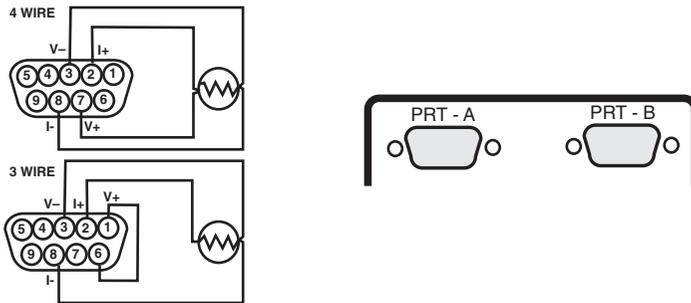
RTDs (Platinum resistance thermometers) must be fitted with a high quality D-plug and connected to input PRT-A and/or PRT-B as required. A 3 or 4 wire configuration can be used but they are connected differently as shown. The instrument will automatically sense which configuration is employed.
