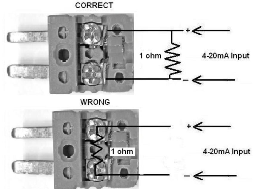
If the input is a 4 to 20mA signal, users can convert the mA signal to mV signal by placing a 1 ohm resistor between two terminals. Then 4mA becomes 4mV and 20mA becomes 20mV.
