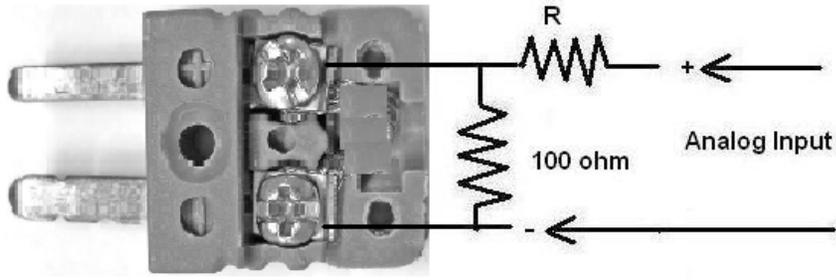
1. If the analog input from an instrument is greater than  $\pm 60\text{mV}$ , users can add two resistors to lower the voltage to less than  $\pm 60\text{mV}$ .
