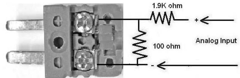
1. The full scale output is  $1000\text{ mV}$  per  $100\% \text{RH}$ .
