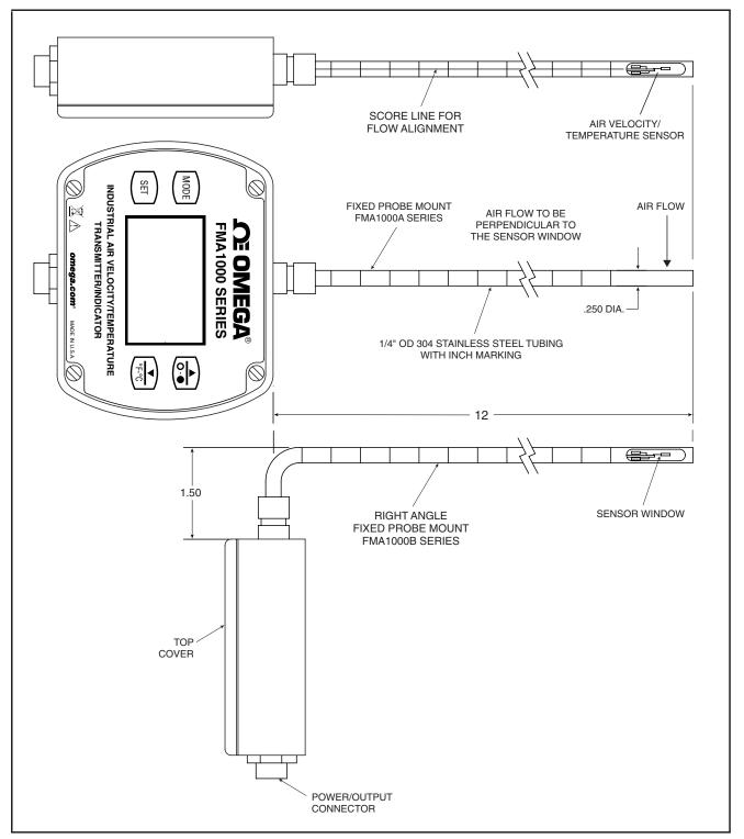
Figure 1. FMA1000 Transmitter with Fixed Probe Mount and Right Angle Mount
