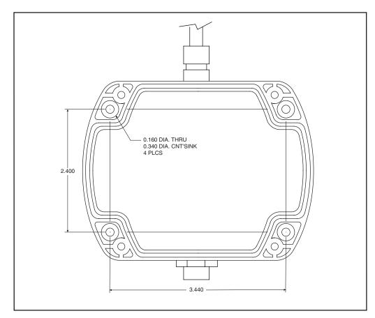
Figure 4. FMA1000 Transmitter Wall Mounting Holes
