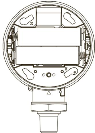
For reattachment of cover, align the 'unlock' icon with the arrow, push cover straight in then turn clockwise until the arrow is in alignment with the 'Lock' icon.
