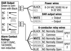
Connect to 8-24 VAC, 50/60Hz or 9-32 VDC. The gauge will operate on either AC or DC power and there is no need to observe polarity. An unregulated power supply can be used. Note that standard 24 VAC transformers with small loads may operate at voltages over the 24 VAC limit. The supply voltage, when within the stated ranges, has negligible effect on the gauge calibration. Operation below 9 VDC or 8 VAC may cause erratic or erroneous readings or output.
