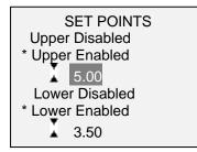
Either one, two, or none of the set points may be enabled. To toggle between the tension and compression directions, press the **DIRECTION** key.
