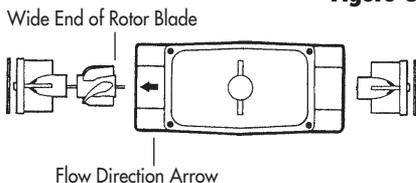
9. Turn the turbine over and drop the second support into place. Put the final retaining ring into position.
