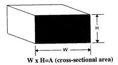
In a circular duct this cross section area equals the radius squared times  $\dot{\pi}$  (3.14).
