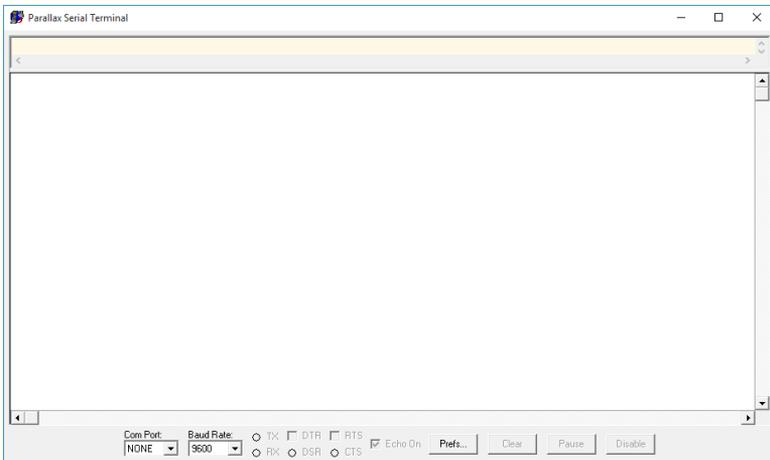
Attach your instrument & probe to your computer via the USB cable. Select the appropriate 'Com Port:'. In the below example, COM5 is being used. Set the 'Baud Rate:' to 9600
