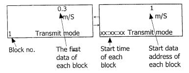
Use ▲ Up Button, ▼ Down Button to select the different data memory block no. ( 1 to 250 ).
