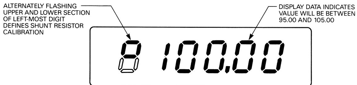
**Figure 5-5. Display Indication for SHUNT RESISTOR Calibration Mode**
