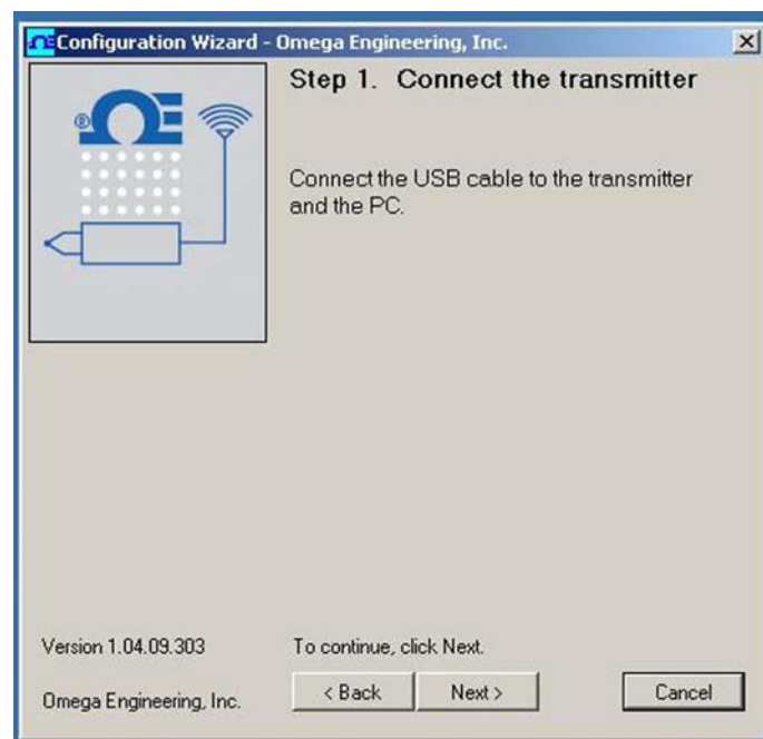
Figure 5-5. Utility Program - Connect To Transmitter Screen
