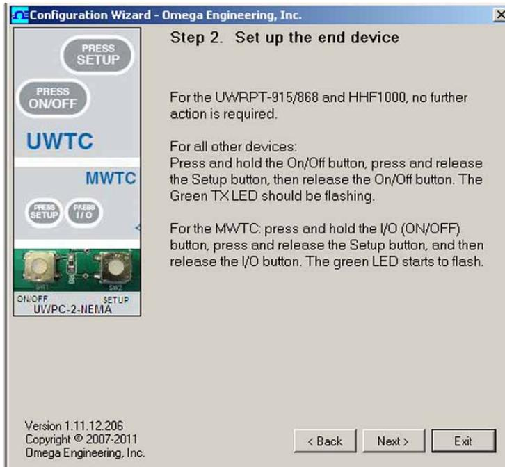
**Figure 5-6. Utility Program - Setup Transmitter Screen**
