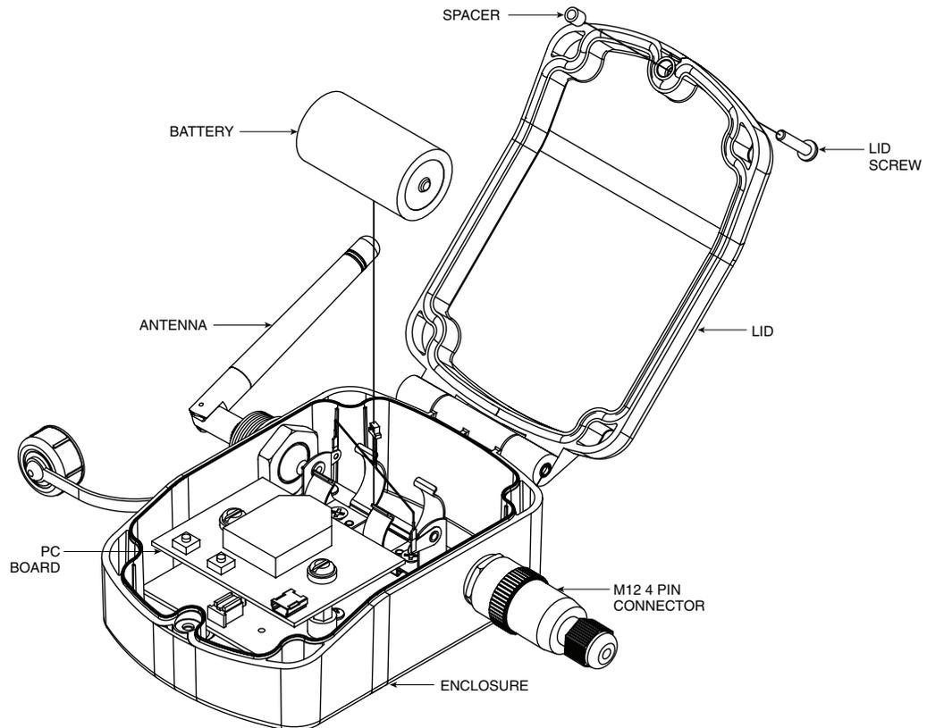
Figure 5-13. Battery Replacement
