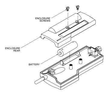
Figure 18A. Battery Replacement, UWRH-2
