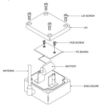
Figure 18B. Battery Replacement, UWRH-2-NEMA
