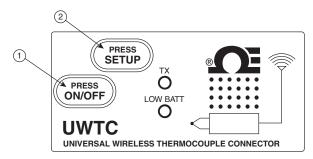
Figure 7-2. Connector/Transmitter Button Operation
