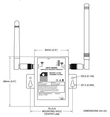
Figure 6-1. Mounting Dimensions
