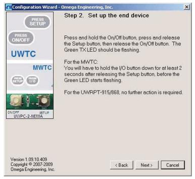
Figure 5-3. Setting Up the End Device
