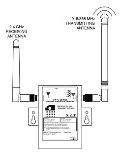
Figure 6-3. Standard Repeater Antennas
