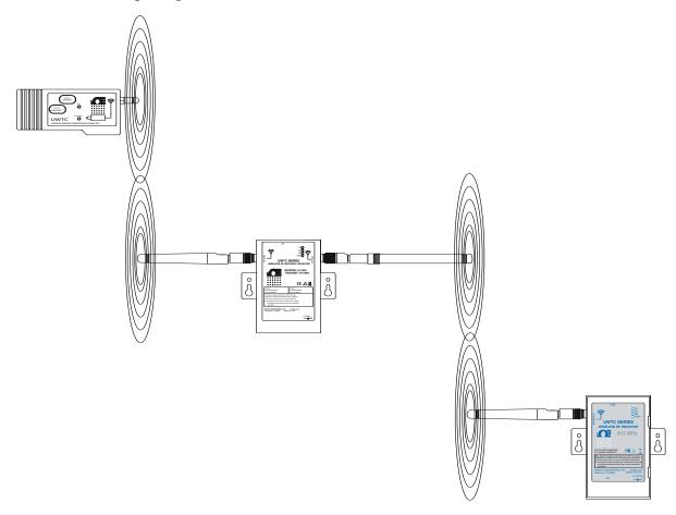
Figure 7-8. Vertical Antenna Placement
