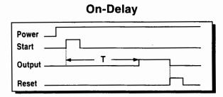
Timing begins on the leading edge of the start input. The output will activate at the completion of the preset time (T) and will remain active until the reset signal is applied or power is interrupted\*.
