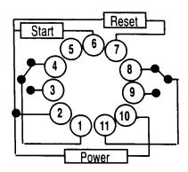
Warning: Do Not connect a coil in parallel with the start signal. Such a connection will cause the start signal to be continuously active. This situation also applies to the Reset input.
