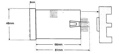
To wire the unit, an 11 pin socket is required. The unit can either be DIN rail mounted or panel mounted using the supplied mounting bracket. For panel mounting, place the unit in the cutout. then slide the bracket forward over the rear of the unit so that the tabs catch in the grooves on the housing and the bracket is as far forward as possible. Tighten the panel mount screws until there is a snug fit against the panel. Do not overtighten.
