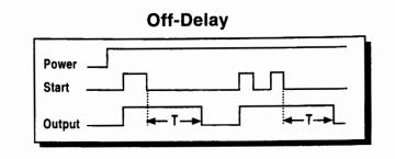
The output is activated at the leading edge of the start signal. Timing begins on the trailing edge. The output will remain active until the preset time (T) has elapsed or power is interrupted\*. Reapplying the start signal before T has elapsed will reset the time value. The reset input is not used.
