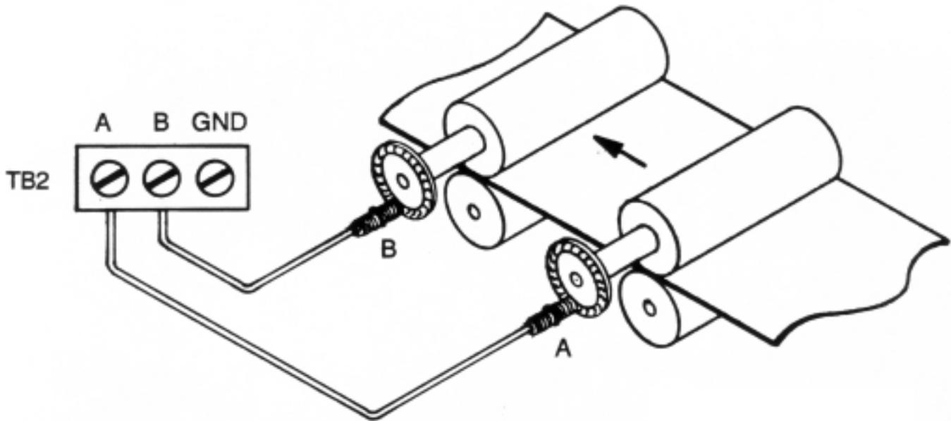
In some applications it is necessary to measure the ratio or draw between two frequencies. For ratio measurement, just program the Function to Fr b/A (frequency ratio B input/A input).
