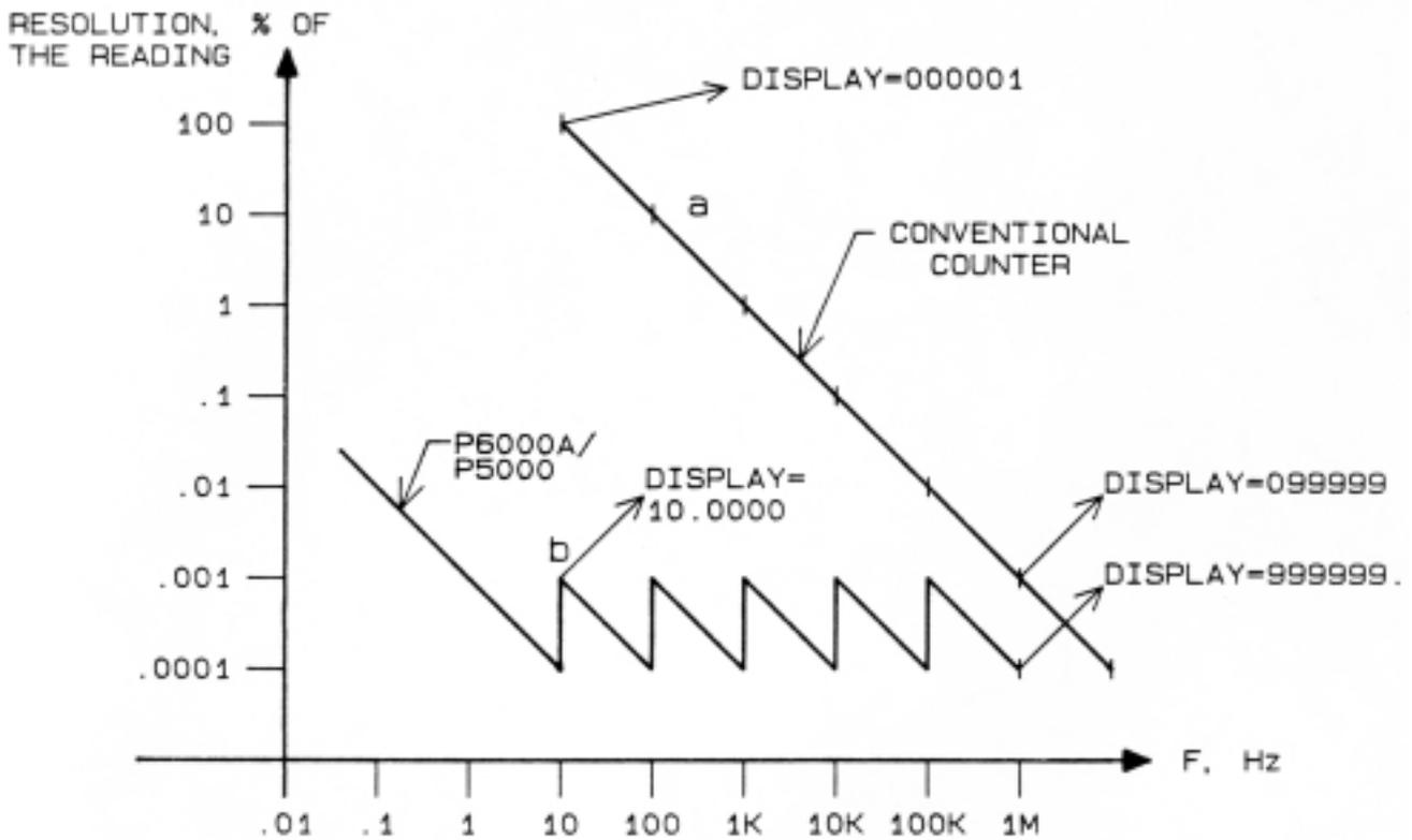
Figure C-1 Resolution Comparison of meter to Conventional Counters
