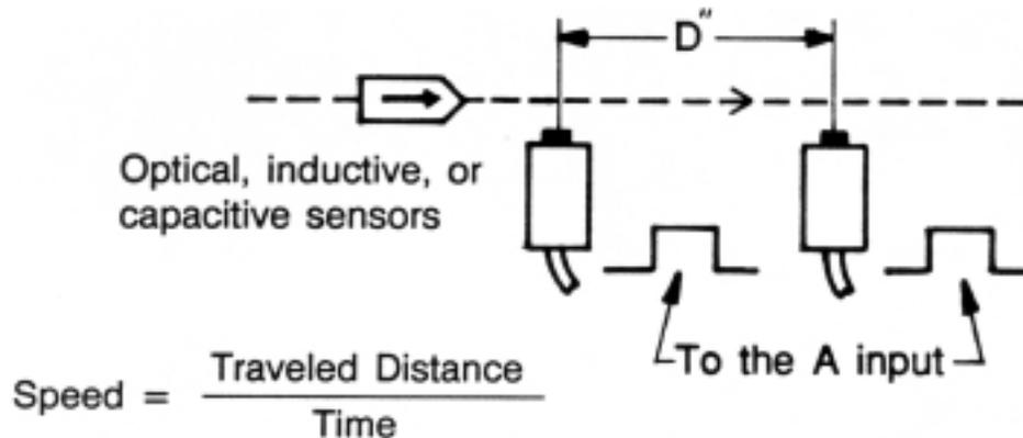
Place two sensors or switches, D inches apart. Use Frequency mode and select zero Gate Time. (The meter will use 2.5 - 3.0 millisecond gate time.)
