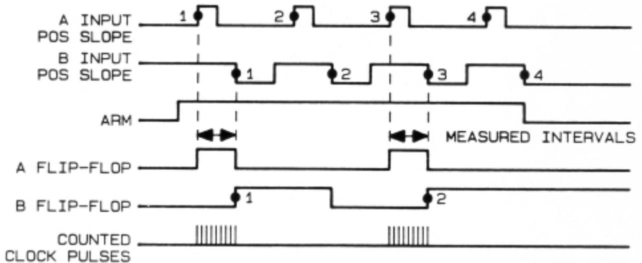
Figure C-3 Time-Interval Measurement Timing
