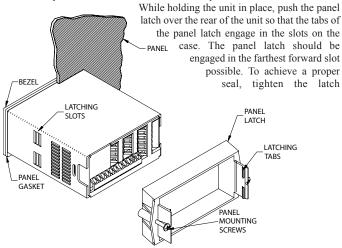
screws evenly until the unit is snug in the panel (Torque to approximately 7 in-lbs [79N-cm]). Do not over-tighten the screws.
