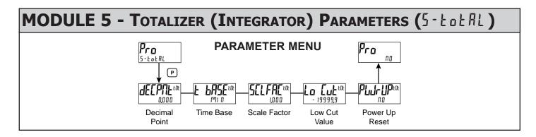
The totalizer accumulates (integrates) the Input Display value using one of two modes. The first is using a time base. This can be used to compute a time temperature product. The second is through a user input or function key programmed for Batch (one time add on demand). This can be used to provide a readout of temperature integration, useful in curing and sterilization applications. If the Totalizer is not needed, its display can be locked-out and this module can be skipped during programming.
