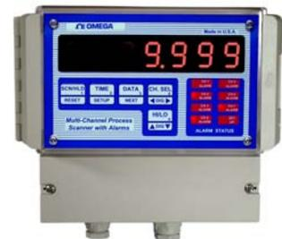
When this parameter is set for "Normally Open", the relay is open when it is deactivated (readings are below LIMIT), and closes when the channel reading exceeds its LIMIT value. When this parameter is set for "Normally Closed", the relay is closed when it is deactivated (readings are below LIMIT), and open when channel reading exceeds LIMIT value.
