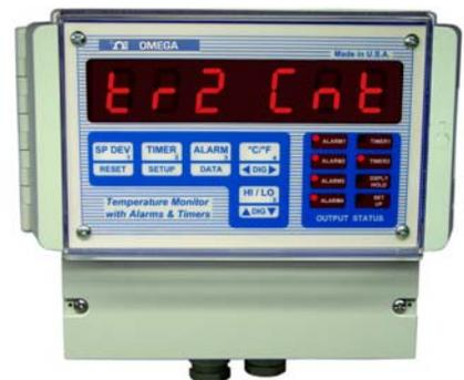
To display Timer #1 value, push the **TIME** key *twice*. The first push shows elapsed time, while the second push will first display 'tr1 Cnt' (for **Timer1** Count) and then Timer 1 value.
