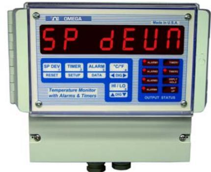
Setpoint value that needs to be tracked can be entered in two different ways. One is during setup mode and the other is using the front key labeled 'SP DEV'. SETUP mode entry is used when a particular value needs to be programmed e.g. 500, 850 and so on. To enter Setpoint in this mode, look under 'SETUP'.
