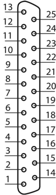
Figure b-1, FMA6600/6700 25 Pin "D" Connector Configuration.
