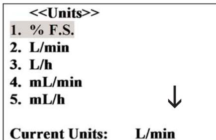
Figure b-4, FMA6600/6700 Units of Measure Screen
