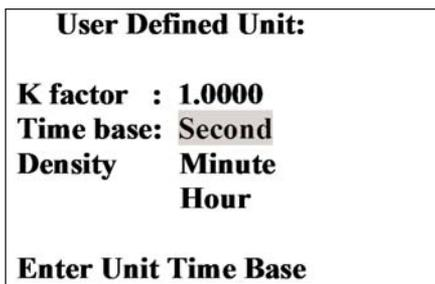
Figure b-6, User Defined Unit of Measure Screen (Time base)
