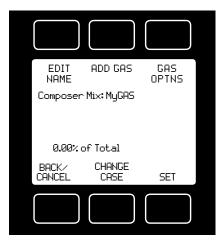
Composer allows you to program and save up to 20 custom gas mixes containing 2 to 5 component gases found in the gas lists (pages 33-40). The minimum resolution is 0.01%.
