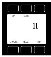
Press **FLOW AVG**. Then use SELECT to choose the digit with the arrow and the UP and DOWN buttons to change the value. Press SET to record your value. Press CLEAR to return to zero.
