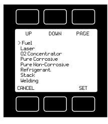
**Gas Select** allows you to set your device to up to 150 standard gases and mixes. You can also use **Composer** to program and store up to 20 additional gas mixes.
