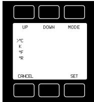
**Gas Temperature:** FMA-1600A flow meters measure the incoming temperature of the gas flow. The temperature is displayed in degrees Celsius (°C). This parameter is moved to the primary display by pushing the button above °C.
