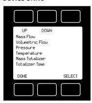
Press **DEVICE UNITS** to access menus of units of measure for each parameter (and totalizer if so equipped).
