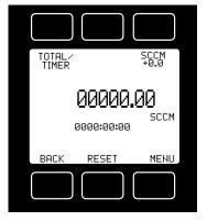
The Totalizing Mode screen is accessed by pushing the TOTAL button on the MAIN display.
