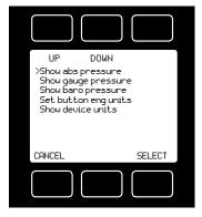
**TARE P w/BARO:** The stream absolute pressure sensor can be tared to the barometric pressure sensor. In this case, the absolute pressure is offset by the differential between the two readings. **TARE P w/BARO** can be accessed from the **MISC2** display.
