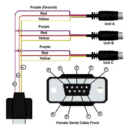
Typical Multiple Device (Addressable) Wiring Configuration
