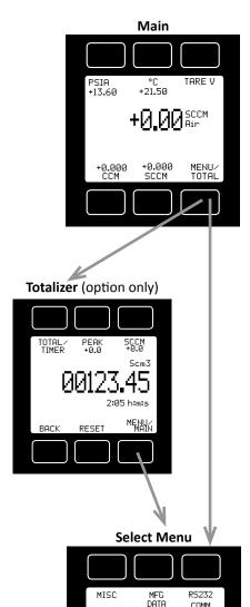
GAS SELECT The Main display shows pressure, temperature, volumetric flow and mass flow.
