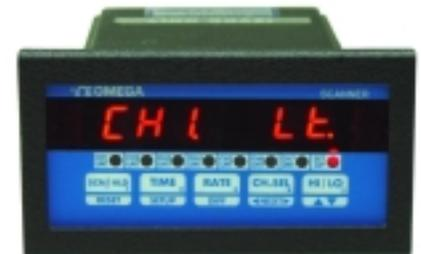
The display will first show '**CHx Lt**' (x=channel #) after which the current LIMIT value will be displayed. Use ^v key (ref. Setup For High Scale) to set the desired LIMIT value. Once the desired LIMIT value is displayed, push **SETUP** key to enter that value and go on to setup Deadband.
