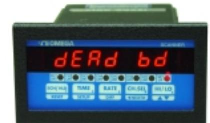
The display will first show '**dEAd bd**' after which present DEADBAND value will be displayed. Use ^v key (ref. Setup For High Scale) to set the desired DEADBAND value. Once the desired DEADBAND value is displayed, push **SETUP** key to enter that value and go on to setup Relay as Normally Open/Closed.
