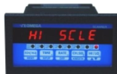
key and then pushing it again will decrement the value (^v key works as a toggle -- alternating between increment and decrement). To change the next digit first push the <NEXT> key. This will advance the flashing to the following digit. Use ^v key to change the value. After the desired High Scale setting is displayed, push **SETUP** key to enter that setting and go to setup Low Scale.
