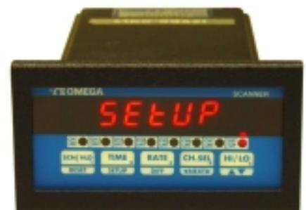
Once the correct pass-code has been entered, the display shows 'SYS CH', with 'CH' blinking. At this point the operator may choose between making channel settings (CH), or system settings (SYS). Use ^v key to toggle between CH and SYS modes. When the desired mode is blinking, press **SETUP** key to begin setup of parameters for that mode. **'SYS' Parameter List**
