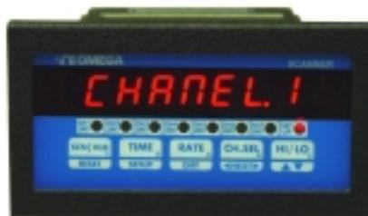
Display time for each channel is programmable from 1-999 seconds (16.65 min.). This is useful for adjusting display time to a rate which is consistent with the type of process being monitored. Scan time for each channel is independent of display time. This permits programming long display times without losing track of the process on other channels.
