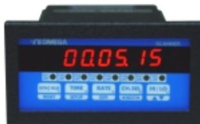
The elapsed time can also be momentarily displayed while the unit is operating in any other display mode. This is done by pushing the TIME key once. The unit will first display the word 'ELPSd t' followed by the elapsed time. This will stay in the display window for a brief period and then the unit will revert to the normal display mode.
