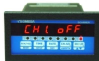
Use **^v** key to display the desired ON/OFF setting, and then push **SETUP** key to enter that setting and go on to setup Decimal Point Position.
