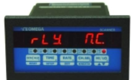
The display will show '**rLy N.O.**' for relay Normally Open or '**rLy N.C.**' for Normally Closed setting. Use ^v key to toggle between the two settings. Once the desired setting is displayed, push **SETUP** key to enter that value and go on to setting up Engineering Units.
