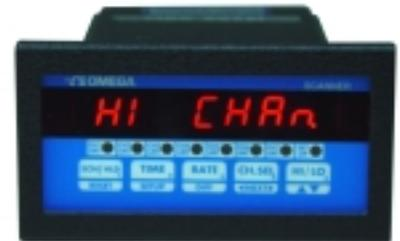
To display high and low channel from any other display mode simply push the **HI/LO** key. Pushing this key once will first display '**HI CHAN**' and then the channel number and the process value will be displayed in the format '**C2 1234**'. The second push on the **HI/LO** key will first show '**LO CHAN**' in the display window, and then the channel with the lowest process value will be displayed.
