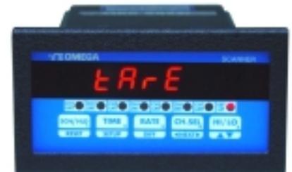
The display will first show 'tARE' after which the current TARE value will be displayed. Use ^v key (ref. Setup For High Scale) to set the desired TARE number. Once the desired TARE value is displayed, push **SETUP** key to enter that value and go to setup Setpoint.
