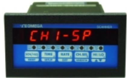
b) The second method of displaying deviation is by selecting the '**dSP dEN**' option when programming the Display Option during the SYS Setup. If this method is selected, the display will scan through all the active channels and display their deviation. The display format is '**d2 1234**' (d stands for deviation).
