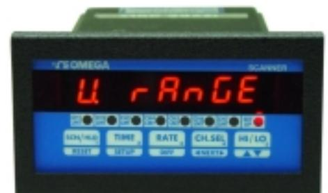
desired value is displayed, push **SETUP** key to enter that value and go to the next step.
