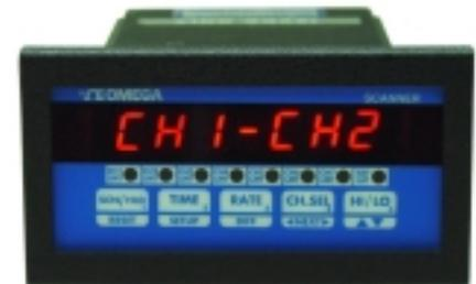
If the unit is not programmed for difference mode, the differential between any two of the seven channels can be briefly displayed by pressing the **DIFF** key.
