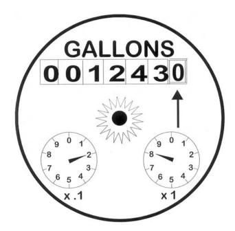
The sample meter reading is 12438.2 gallons. The single gallon counter is on the right hand corner (small dial) and shows indication x1. The fraction of gallons is indicated on the left side of the dial indication that each number adds .1 gallon.
