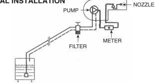
Meter should always be in lower position than the nozzle to prevent the oil from flowing out of the meter.
