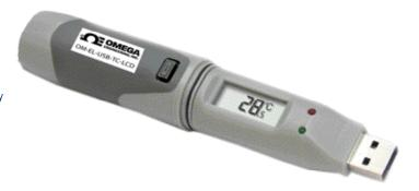
This standalone data logger measures and stores up to 32,510 temperature readings from either a K, J or T type thermocouple. A thermocouple is attached via the thermocouple socket at the base of the unit. The user can easily set up the logging rate and start-time, and download the stored data by plugging the data logger into a PC's USB port and running the purpose designed software under Windows 2000, XP, Vista or 7. Data can then be graphed, printed and exported to other applications.
